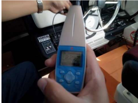
Pre-addition idling 500rpm Vibration level : 2.25m/s 2
