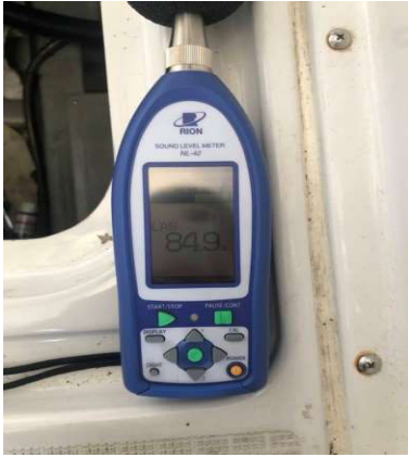
Pre-addition at 1,500rpm Noise : 84.9dB
