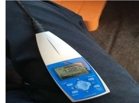
Post-addition idling 600rpm Vibration level : 1.22m/s 2
