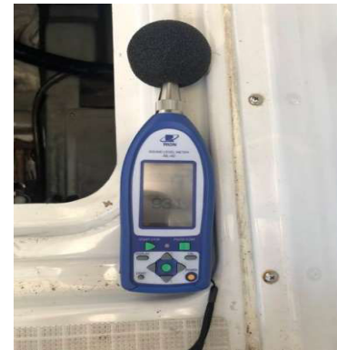
Post-ad 2,000rpm Noise : 93.1dB
