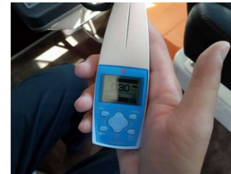
Post-addition engine at 1,000rpm Vibration level : 0.30m/s 2
