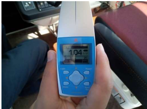
Pre-addition engine at 1,000rpm Vibration level : 1.04m/s 2
