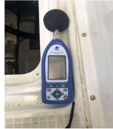
Post-addition at 1,500rpm Noise : 84.1dB
