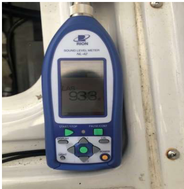
Pre-ad 2,000rpm Noise : 93.3dB
