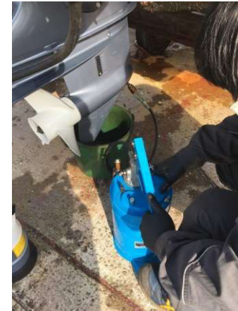
Inject using pump
