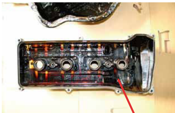
Removing head cover exposes carbon sludge on camshaft and engine
