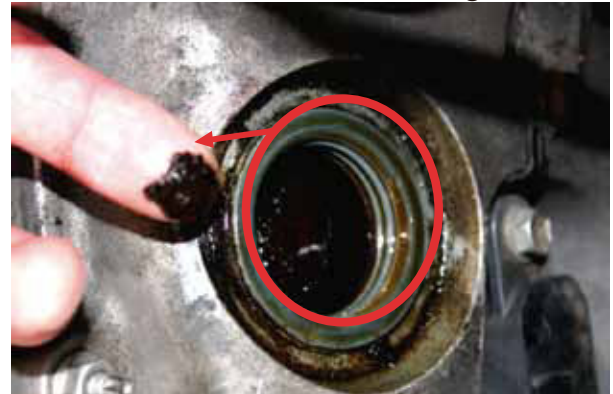
Sludge-like oil residue
