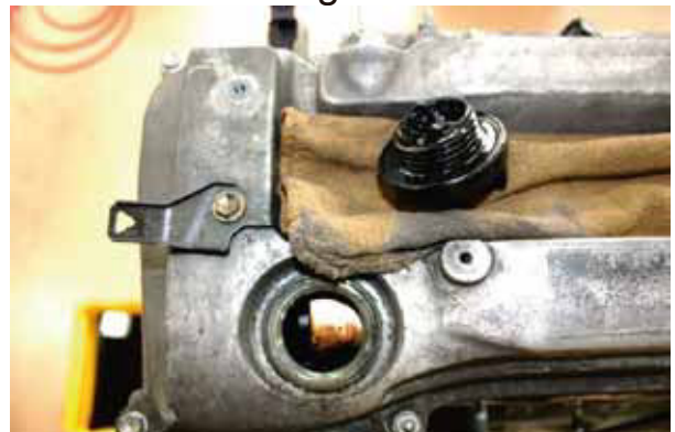
Sludge on filler cap, but not around oil vent due to vehicle type.
