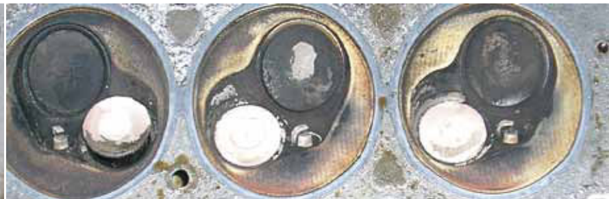
Carbon almost gone from combustion chamber Improved compression, clean chamber from optimum combustion
