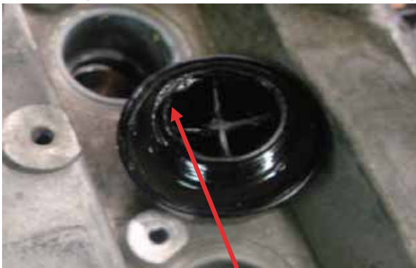
Sludge on filler cap, but not around oil vent due to vehicle type.
