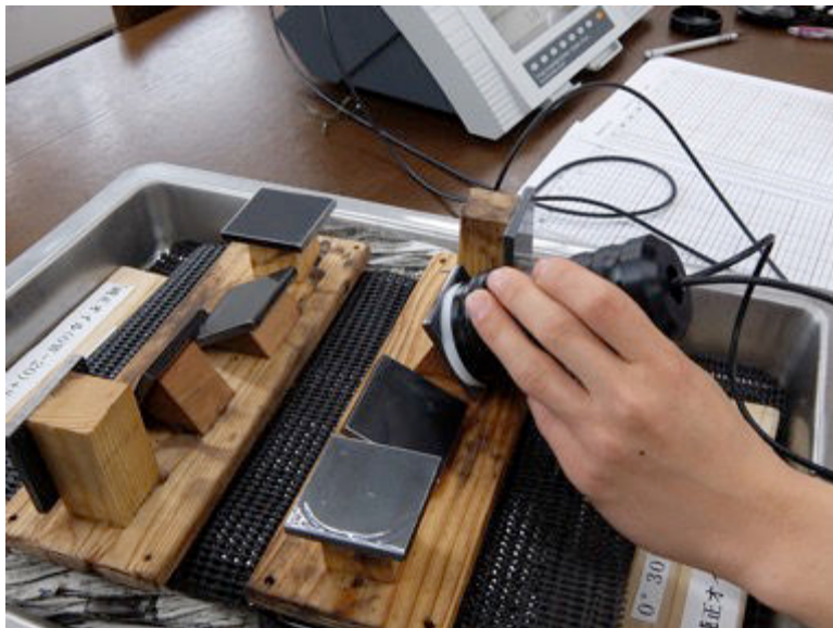
Measuring the plates with a beta emitter to measure the oil film thickness in microns
